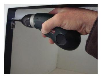
2. Position the Fascia Assembly into position with the female clips attached correctly. Once it is in its correct position (see Cabinet Specifications in this manual), screw the female clips into position using the 6 gauge screws provided.
