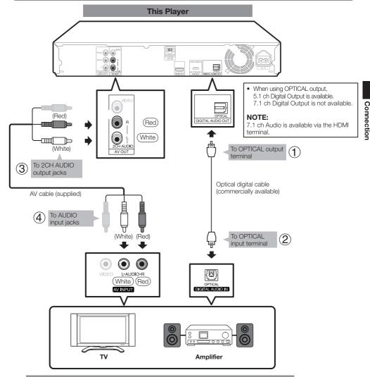
Audio equipment with a digital audio input terminal or audio jacks
