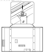
2) Attach the eye bolt connection plate (upper) and secure in place with the eye bolt used in step 1).
