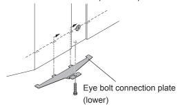
8 Confirm that the LCD Monitor is mounted securely, and then remove the hooks of the hoisting device.
