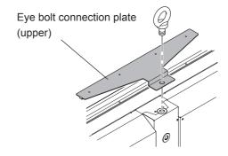
Insert the hooks of the hoisting device into the eye bolts of the protection panel and slightly lift the panel.
