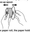
7. Install a new paper roll, the paper holding plate and the take-up spool according to the instructions in "Getting Started."
