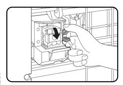
Hold the staple box release lever to unlatch the staple box.
