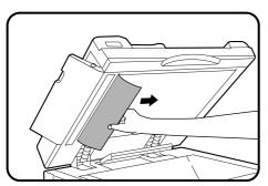
(C) Open the feeding roller cover and the document feeder cover, and remove the original.
