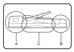
An original misfeed may occur at one of three locations: (A) in the RADF feed section, (B) in the exit roller, or (C) under the transport belt.
