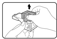
Remove the empty staple cartridge from inside the staple box.
