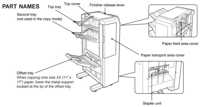
• The top tray and second tray are each furnished with an extendable component, which is to be used when copying onto size A3 (11" x 17") paper.
