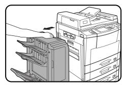
While holding the finisher release lever, slide the finisher away from the copier.
