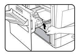
(3) Remove the misfed paper from the section below the exit area.
