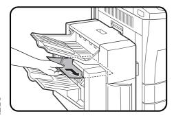
Insert a new sheet of paper (A4 or 8-1/2" x 11" size) to the tray as shown in the picture to make the stapler work properly.
