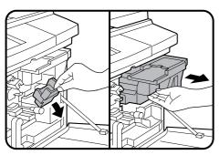
Pull down the toner hopper lock lever and pull the toner hopper out slowly until it stops.
