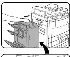
While holding the finisher release lever, slide the finisher away from the copier.
