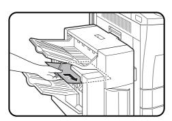
Insert a new sheet of paper (A4 or 8-1/2" x 11" size) to the tray as shown in the picture to make the stapler work properly.
