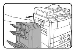
While holding the finisher release lever, slide the finisher away from the copier.
