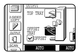
In the initial setting, the offset tray will move from side to side so that each copy set is offset by approximately 30 mm (1.2 inch).
