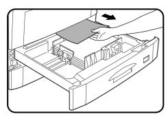
If the paper cannot be seen from the side, pull out the paper tray which was in use and remove the misfed paper.
