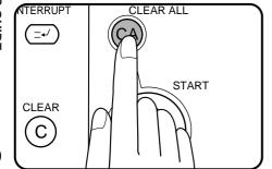
To exit the key operator program mode, press the CLEAR ALL (((A)) key.
