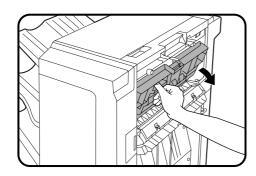
3 If the misfed paper cannot be removed in step 2, open the cover of the paper feed area of the finisher.
