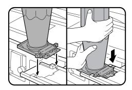
Place the new toner cartridge with the tabs in the notches as shown.
