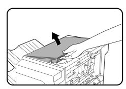
5 If the misfed paper cannot be removed in step 4, close the cover of the paper feed area and open the top cover.
