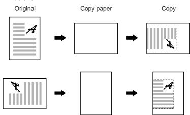
To enable rotation copy, press the check box of "ROTATION COPY SETTING." to display a check mark in the check box. To disable this mode, press the check box of this program again to clear the check mark in the check box.
