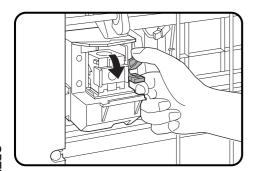
Hold the staple box release lever to unlatch the staple box.
