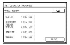
The total counts for all units in use will be displayed. To print these counts, press the "PRINT" key. Press the "OK" key to exit the program.
