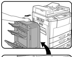
While holding the finisher release lever, slide the finisher away from the copier.
