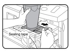
Hold the toner cartridge with one hand while pulling on the sealing tape to remove it.
