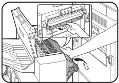
Rotate the paper feed area cover as shown to open it.
