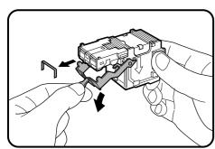
Lower the lever at the end of the staple box and remove the jammed staples.
