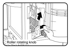
• If the misfed paper is not seen in the paper transport area, turn the roller rotating knob to feed the paper.
