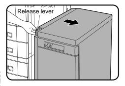
While holding the tray release lever, carefully slide the large capacity tray away from the copier until it stops.
