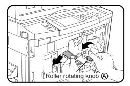
2 Turn roller rotating knob (A) in the direction of the arrow to remove the misfed paper.
