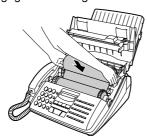
Wind the film slightly (rotate the gear on the right side of the rear spool) so that there is no slack in the film. Make sure that both edges of the film wind onto the spool evenly.
