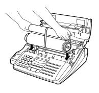
5 Cut the band which holds the spools together with scissors, and remove it. Insert the remaining gear into the right end of the empty spool and the flange into the left end of the empty spool. Make sure the tabs on the gear and the flange fit into the slots in the ends of the spool (the gear has two tabs and the flange has one tab).
