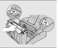
**5** Place your thumb on the center of the handle where it is marked PUSH, and push the handle down and in so that the cartridge fits into place.
