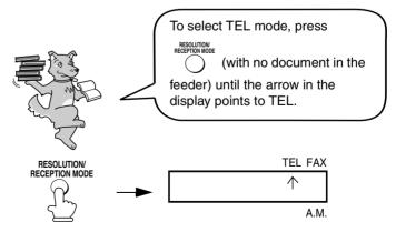
When the reception mode is set to TEL, you must answer all calls (even fax calls) by picking up the fax machine's handset or an extension phone connected to the same line.
