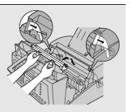
**6** Replace the toner cartridge and close the print compartment cover (see page 15). When finished, reset the drum cartridge counter as explained on page 18.
