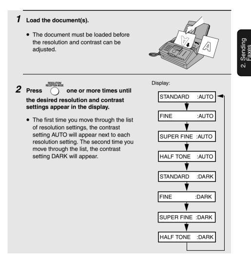
**Note:** In order to transmit in SUPER FINE resolution, the receiving fax machine must also have that resolution. If it doesn't, your machine will automatically step down to the next best available setting.
