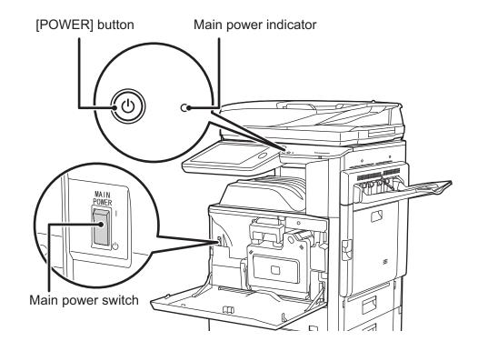
When using the fax or Internet fax function, always keep the main power switch in the " | " position.
