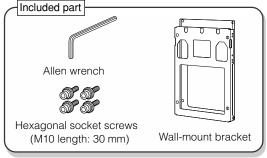
Use an Allen wrench to screw in the included hexagonal socket screws into the Mark A holes.
