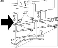
Removing the edge covers reveals the stand fastening screws in the center of the stands, so remove these screws.
