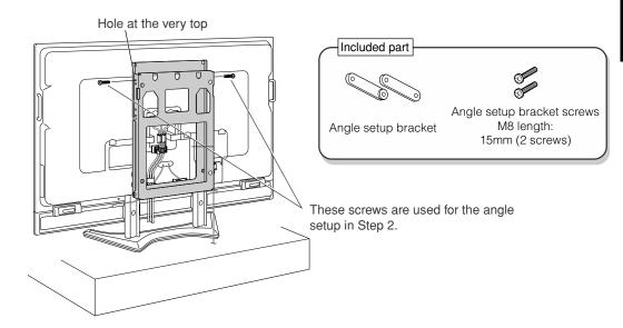
Assemble the included angle setup brackets as shown in the illustration and then use them to set the TV to the desired angle.
