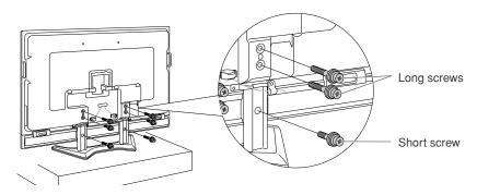
(1) Remove the 2 screws from each of the stand edge covers (total of 4 screws from the left and right sides).
