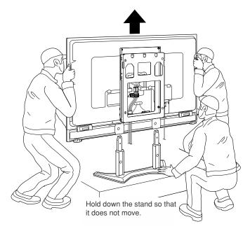
Temporarily place the LCD color TV on a cushion or soft material and install the stand hole covers that are included with the LCD color TV.
