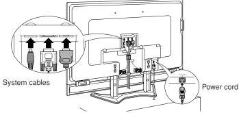
Use the cable holder at the center of the back of the LCD color TV and the cable holders holding the speaker cables to connect the system cables.
