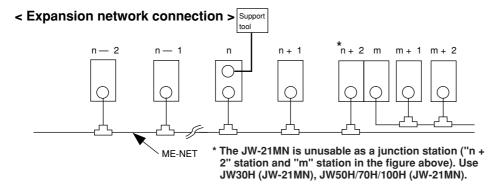
The operations below using a peripheral device, that is connected to a "n" station, is possible.
