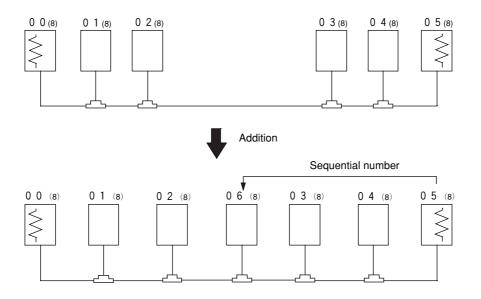
$\geqslant$  means the termination resistance switch being turned "ON."
