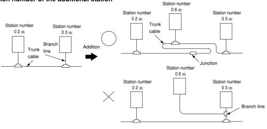
Station number of the newly added station should be next largest number from the current largest numbered station. Each station should not be required to be arranged in order of each station's number.
