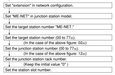
Set the installed slot number of the master station on the target station side. In the case of the above figure: 3.
