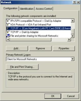
Step 3 In the Configuration tab, you can see several network components under The following network components are installed: Make it sure that a network adapter connected with AHT-E300 ADSL Router appears in the list of the network components.
