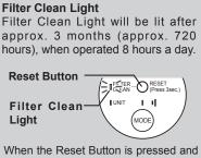
When the Reset Button is pressed and held in for at least 3 seconds, the light flashes twice then turns off.
