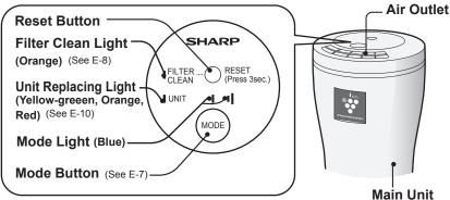
The Unit Replacing Light is always lighting during operation.
