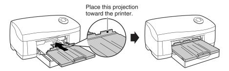
**7** Pull out the output tray extension to the proper position, and then raise the paper stop guide.
