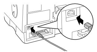
**3** Insert the other end of the cable into the interface connector of your computer, or the USB hub connected to your computer.
