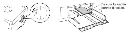
2) Set guide (3) up, and then fit guide (1) and (3) against the loaded cards.
