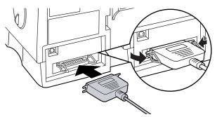
4 Insert the other end of the cable into the interface connector of your computer.
