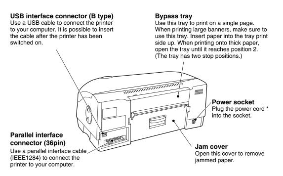
\* When the power cord is connected to the outlet, power for the printer is turned on automatically.
