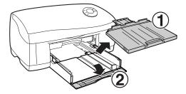
**2** Adjust the guides ① and ② shown in the illustration to the width of the paper.
