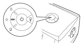
If the ink lamp continues to blink, open the front cover, return to step 5 of "Installing the Print Head" and follow the procedures once more.
