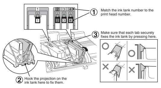
Make sure that the numbers on the ink tanks correspond to the numbers on the print heads. If they do not correspond to each other, print problems will occur. In this case, replace the ink tanks to the correct positions, and then print a test page referring to "Test Print Head" in the Online Manual. Before sending any print job to the printer make sure that the test page is successfully printed.
