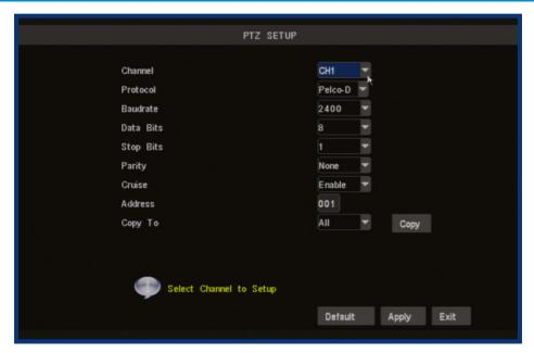
This is where you configure the DVR to act as the controller for a PTZ capable camera system. PTZ devices are connected via the RS485 connection on the rear of the DVR. You'll need the manufacturers documentation for your PTZ system on hand to correctly set it up. The DVR is not compatible with all PTZ systems - in these cases, you'll need a stand-alone PTZ controller.
