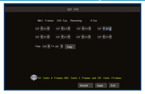
**Frame Rate:** How many frames per second (FPS) the DVR records. "Real-time" is 25 fps (PAL) or 30 fps (NTSC). However, even lower frame rates are okay - even 3fps is still the equivalent of three photographs per second.
