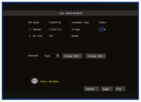
This is the **HARD DRIVE (HDD) MANAGEMENT** screen. All aspects of the hard drive can be managed from this screen.
