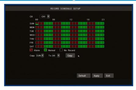
In this example image, the CH1 will record only ALARM events between midnight and 3:00AM, CONSTANTLY between 3:00AM and 6:00AM, then continue to alternate between alarm events and constantly recording for the remainder of the day.
