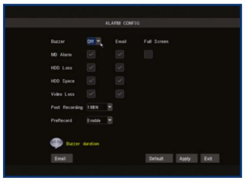
From this menu you can configure the DVR to emit an alarm tone from it's internal buzzer, or configure the DVR to send an 'Auto-Mail' email alert when motion is detected.
