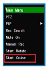
To setup CRUISE MODE, you'll need to define "POINTS" for each channel with a PTZ camera you want to "cruise". A POINT is one place that the camera needs to move to on its loop.
