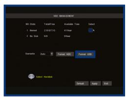
**Above:** The **HDD Managment** menu, with the **FORMAT USB** button highlighted.
