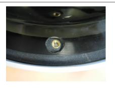
9. Align the dome cover and dome ring over the holes. (See image above)
