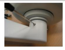
Fix the wall mounting bracket onto the dome by screwing in the 3 holding screws in a clockwise direction using a flat head screw driver.
