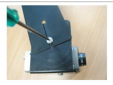
Adjust the camera bracket to suit your viewing direction. Then secure the bracket into place by screwing the locking screw in a clockwise direction.
