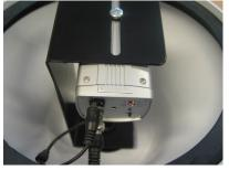
7. Connect the AV and DC cable onto the back of the camera. This illustration shows how to connect the cables into the back of a Swann C500, but actual connections will vary depending on your camera.
