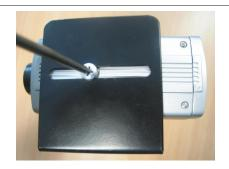
1. Firstly attach the camera onto the camera bracket. Keep the orientation of the dome in mind when mounting the camera.
