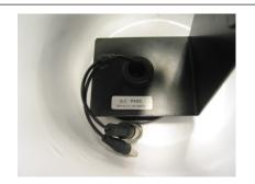
5. Now thread the cable into the bottom of the dome.
