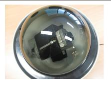
10. Secure the dome cover to the dome body using 3 screws supplied.
