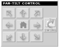
When you connect a pan/tilt camera, the system will detect the camera's function automatically and the PAN-TILT CONTROL buttons will become functional. Otherwise, these buttons are displayed as grayed out buttons.
