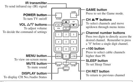
You can test if the remote control sends out the infrared signal with an AM radio.
