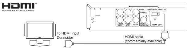
A display equipment with an HDMI compatible port
