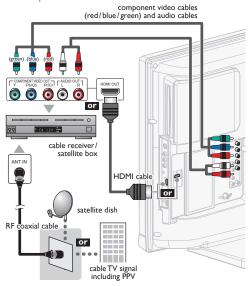
You can also connect this unit to the cable receiver or satellite box other than the HDMI or the component video output jacks because they might have different output jacks.
