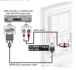
Use an HDMI cable with the HDMI logo (a certified HDMI cable). High Speed HDMI cable is recommended for the better compatibility.
