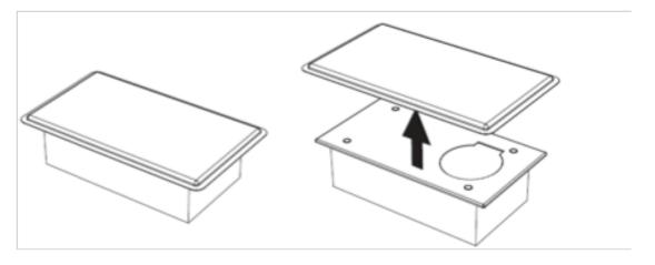
Step 2: Remove cover plate by first removing the screw caps and then unscrewing the screws. Save screws.
