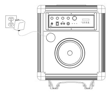
Plug the included AC/DC power adapter (120W/60Hz 15V) into the DC POWER INPUT on the dock and an AC power outlet to power the dock.
