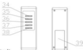
Insert (2) "AAA" 1.5V batteries (not included) following the polarity as indicated in the compartment to the right. Alkaline batteries are recommended for long using time.
