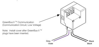
Dimming Interface (galvanically isolated) for controlling 0-10V electronic dimming ballasts (30mA maximum sinking capability). Relay Contact (Line Voltage) switches electronic ballasts; recommended relay switching capacity 347V, 20A maximum
