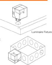
GreenBus II<sup>™</sup> communication wiring is still accessible from the outside of the fixture, while all necessary wiring to the electronic dimming ballast is available on the inside.
