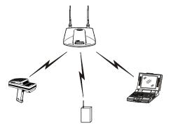
A single AP can bridge the Ethernet and radio networks.
