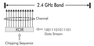
Only 3 non-overlapping Channels of Direct Sequence information fit into defined 2.4 GHz band.
