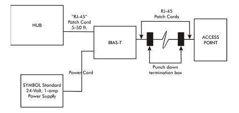
To install a BIAS-T system using a single BIAS-T unit and access point:
