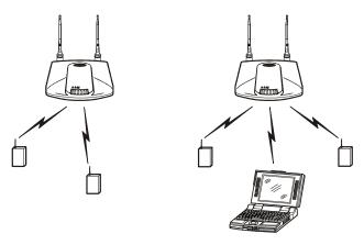
Multiple APs wired together provide a network with better coverage area and performance when using the same Net\_IDs.
