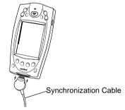
2. Plug the power cable into a wall outlet and plug the other end into the battery charging receptacle on the side of the syn-chronization cable.
