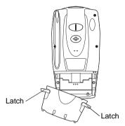
Insert the lithium-ion battery in the battery compartment with the battery tether positioned properly (as shown below), making sure the battery snaps into place.
