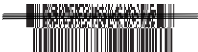
Aim the single scan line at the center of the 2D portion
