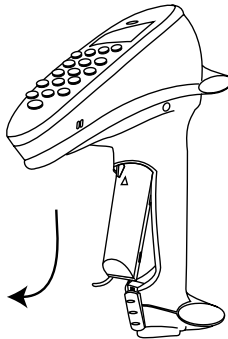
Figure 4-2. Pulling the Battery Out
