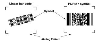
2. Hold down the scan button until the imager beeps, indicating the bar code is decoded.
