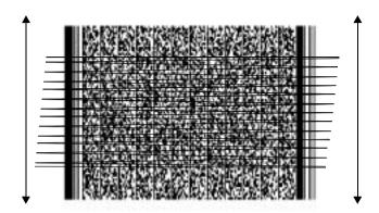
The scan beam does not have to be *perfectly* parallel with the top and bottom of the symbol (up to a 4° tilt will work).
