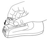
If the battery latch is not closed, do not operate the terminal, otherwise data may be lost.
