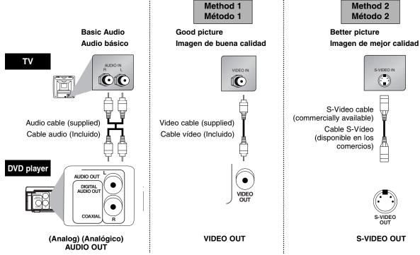
• Connect this unit directly to the TV. If the A/V cables are connected to a VCR, pictures may be distorted due to the copy protection system.
