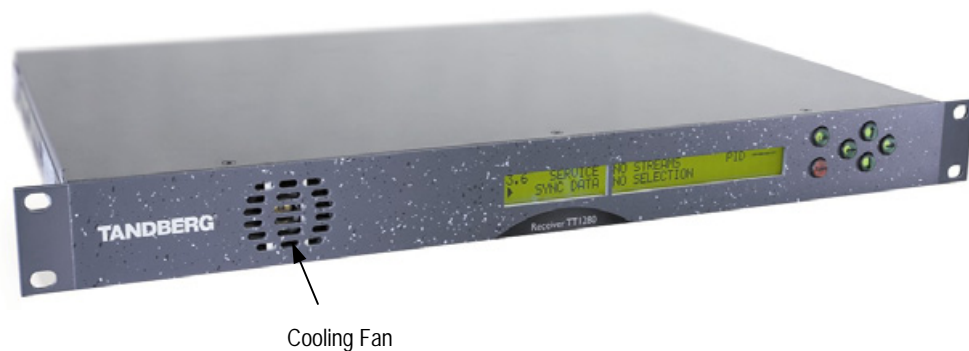
Figure 7.1: Cooling Fan Location
