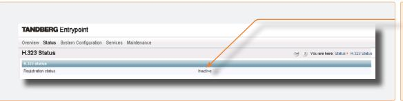
In case the Entrypoint is in direct mode or in case the gatekeeper IP address is filled in incorrectly, the Entrypoint will not be registered with the Gatekeeper, and the Registration status is stated as Inactive.
