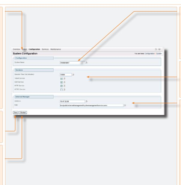
Configuration. To change the system name of the Entrypoint, enter the new system name in the System Name field.
