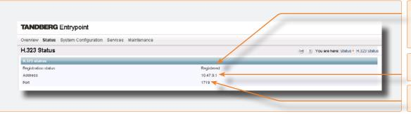
Registration Status. If Registered, the Entrypoint is registered to the Gatekeeper with below mentioned Address and Port.
