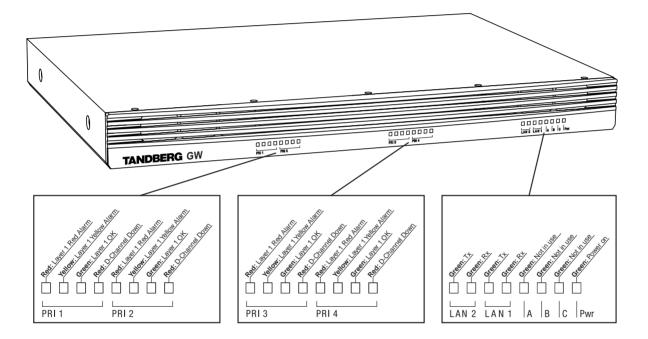
**Red Alarm** or Loss of signal (LOS) indicates that there is no signal and thus no framing info received. The same effect will be obtained by pulling out the PRI cable. This may also be caused by a broken connector in the receive (RX) part of the cable.
