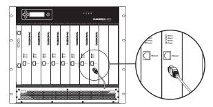
Connect a LAN cable from the Ethernet socket of the board just installed and to your network.
