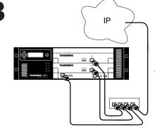
Connect a LAN cable from the Ethernet socket of the board just installed and to your network.
