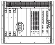
Use the rear panel power switch to switch off the MPS power.
