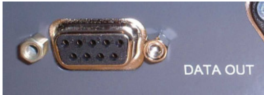
Figure 5.5: High Speed RS-422 Data Enabler Card Rear Panel
