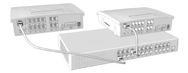
Connect up to four TalkSwitch units (2 are shown in this illustration) to the LAN switch or switched hub.
