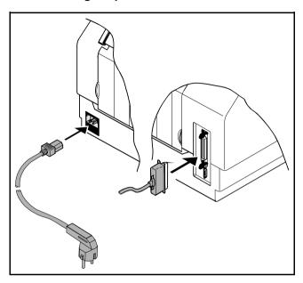
Make sure that the printer and the computer are switched off and connect the data cable between the printer and the computer. Connect the power cable to the power inlet of the printer. Connect the power cable plug to a mains socket.
