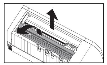
Raise the printer bar cover and remove the used cassette.
