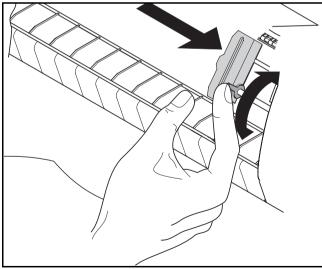
Close the tractor flap and slide the tractor to the right until the paper is slightly tensioned.
