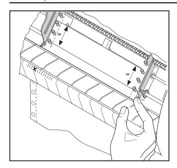
Align the right-hand tractor to the width of the paper and insert the paper. Make sure that it is inserted by the same length as on the left-hand tractor in order to avoid any paper jam.
