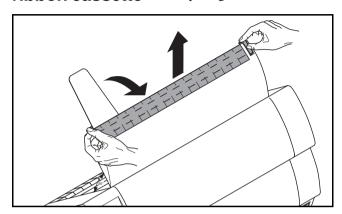
Press the two slide latches, raise the top cover to an angle of 90 degrees relative to the top cover of the printer and remove it.
