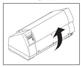
You can set the printer to the correct mains voltage yourself. To do this, cautiously place the printer on its back side.
