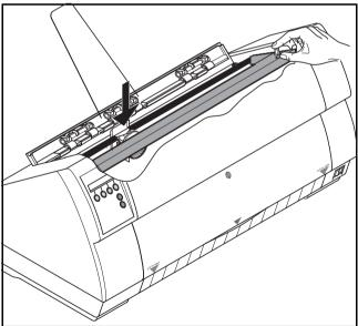
Use the knob on the right side of the cassette to take up slack of the ribbon again. Thereby the ribbon will slide over the plastic noses on the left and right of the print head into the correct position.
