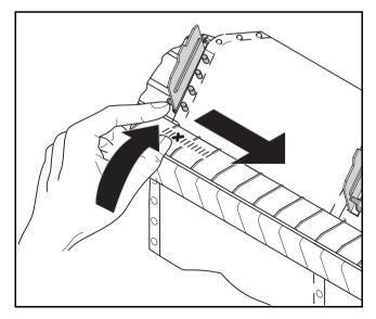
First insert fanfold paper into the left-hand tractor. Make sure that at least three paper transport holes are positioned on the tractor pins. Close the left tractor flap.
