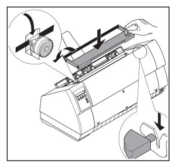
Turn the coloured ribbon feed knob at the right of the new ribbon cassette in the direction of the arrow in order to take up slack of the ribbon.
