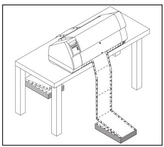
If you expect that frequent forward and reverse feeds will occur, you should place the printer as shown in the figure, if possible.
