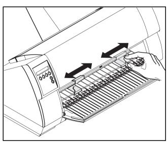
Align the left paper guide with the mark on the left of the single sheet input tray. Adjust the right paper guide to the width of the paper used.
