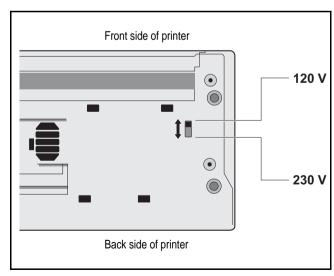
Use a suitable object (e.g. a screwdriver, but never a pencil) to set the slide switch on the left at the bottom of the printer to the correct voltage.
