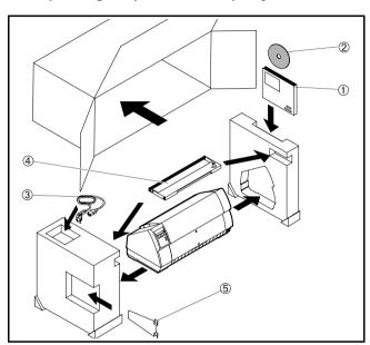
Open the packaging and take out the ribbon cassette. Pull the printer out of the cardboard box towards you and remove the remaining packaging material.
