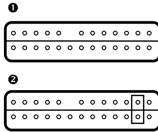
Figure 3-4 Positions de Cavalier TRM PWR
