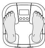
Heels centered on electrodes
