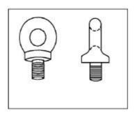
The i15 is flown by using high quality M8 eyebolts with collar to BS4278: 1984. These eyebolts are supplied as part of an optional flying kit and come in packs of three. The i15 is equipped with internal steel braces which also double as the flying points accepting the M8 eyebolts.
