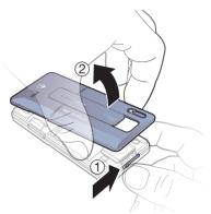
1 Slide and hold the clasp sideways and remove the battery cover.
