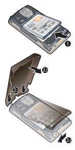
1 Insert the battery with the label side up and the connectors facing each other.
