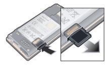
Open the cover and press the edge of the memory card to release and remove it.
