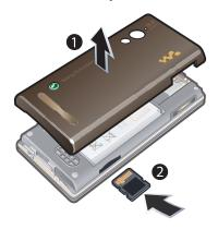
Open the cover and insert the memory card with the gold-coloured contacts facing up.
