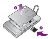
· Remove the battery cover and insert the memory card with the gold-coloured contacts facing up.
