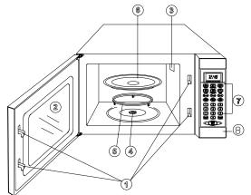
Door Safety Lock System Oven Window Oven Air Vent Shaft Roller Ring Glass Tray
