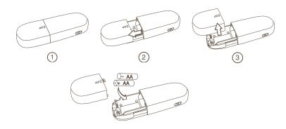
• Slide the battery cover back into position
