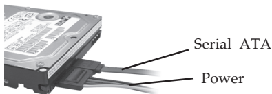
Figure 2: SATA hard disk drive connections
