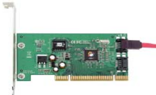
Figure 3. Connecting the Serial ATA data cable
