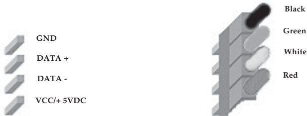
Figure 2. USB Pin-out Header
