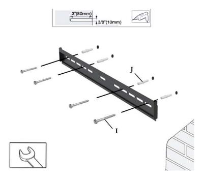
**CAUTION:** Do not over-tighten bolts - doing so may cause unnecessary damage to the wall. **CAUTION:** Do not release the wall plate until it is properly mounted and secured to the wall.
