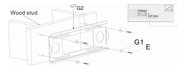
**CAUTION:** Do not over-tighten bolts-doing so many cause unnecessary damage to the wall. Avoid excessive torque.
