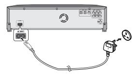
Wall socket (AC 220 V- 240 V, 50 Hz)
